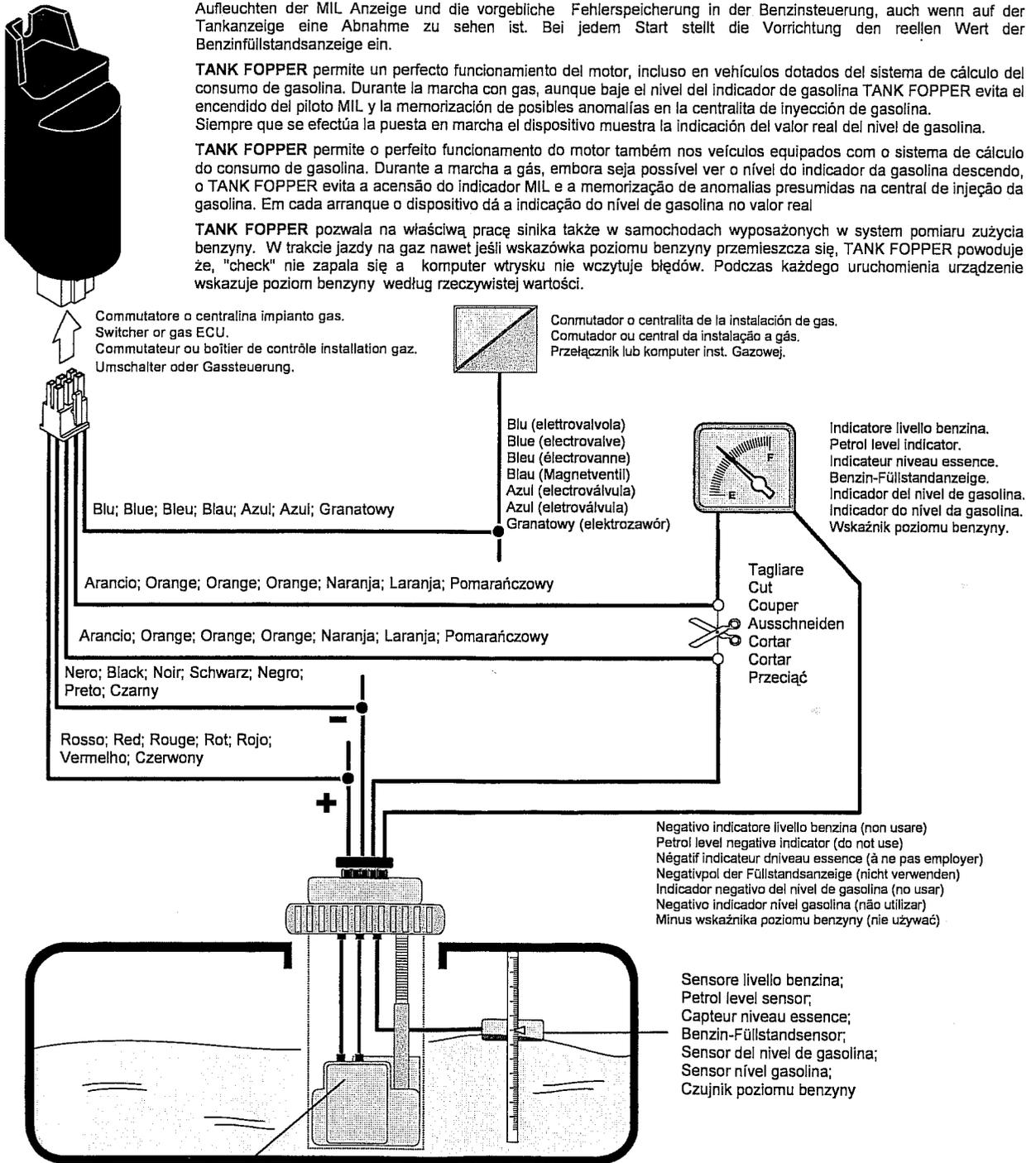
Elettropompa benzina; Electric fuel pump; Electropompe essence;
