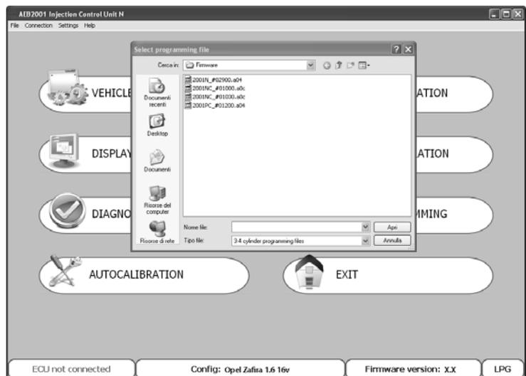
**NOTE:** To avoid losing the configuration of the control unit, make sure that the control unit is connected to the computer before updating. Whether or not the control unit is connected is indicated on the bottom left-hand side of the main menu screen.
