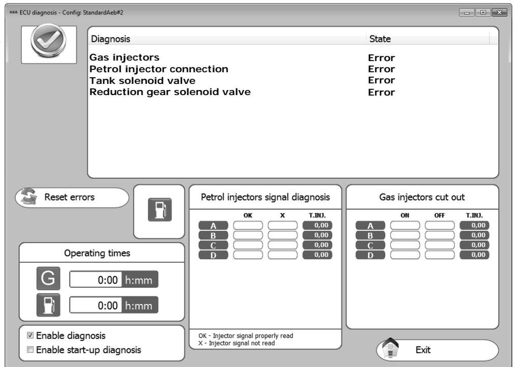
When the GAS control unit detects a diagnosis error on the parameter read, it will perform the action corresponding to the error detected. The possible diagnoses of the PETROL control unit are:
