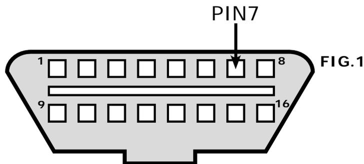
Connect the GREEN wire to the signal found on PIN 7 of the OBD connector.
