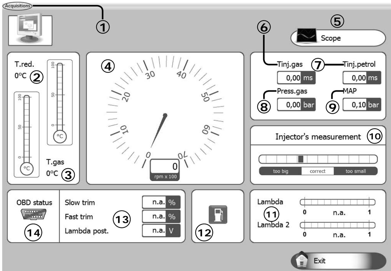
**1) Acquisitions:** For storing the GAS control unit operation parameters in a file that can be displayed via a chart.
