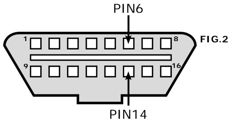
Connect the YELLOW-GREEN wire to the signal found on PIN 6 and the wire YELLOW-GREY to PIN 14 of the OBD connector.
